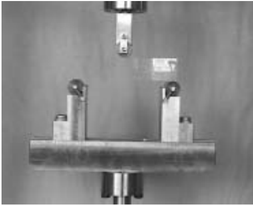
Fig. 3 Set up of three point bend specimen in testing machine
